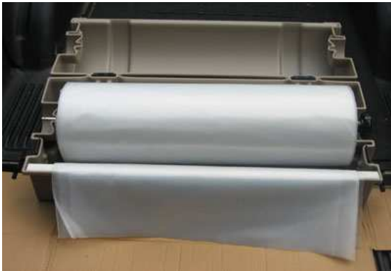
5. Lift roll by spindle ends and set into the Ypod's spindle supports.
